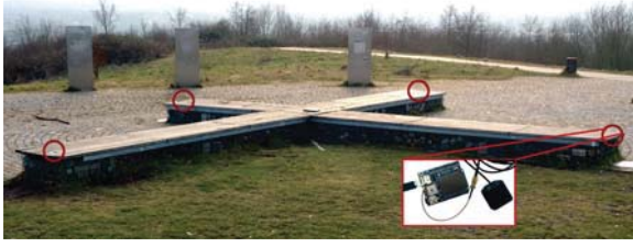
Figure 3: Setup of a central laptop connecting four receivers positioned on each end of a wooden bench (red circles).
