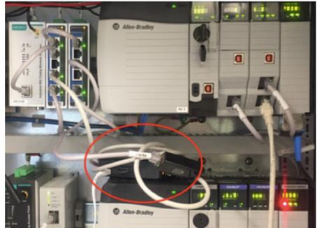
**Fig. 7.** Raspberry Pi3 connected between PLCs.
